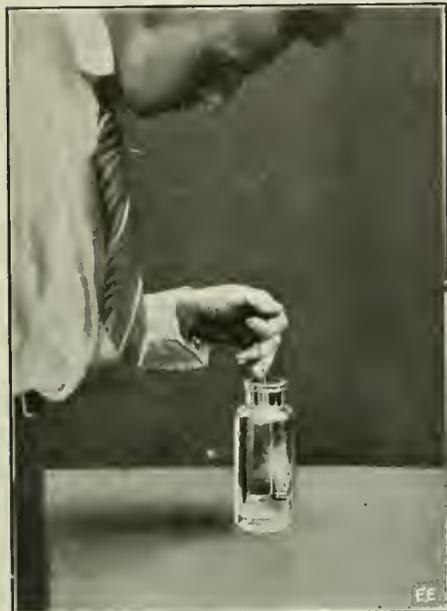
Fig. 81. Introducing Burning Sulfur In Bottle for the Minute Preparation of Sulfuric Acid—H<sub>2</sub>SO<sub>4</sub>.
